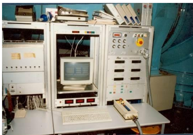
Figure 7-c the six component balance data acquisition system and the speed control system of the wind tunnel
