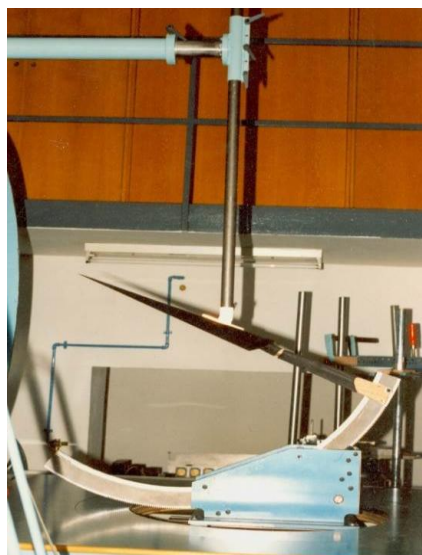
Figure 7-a: The delta wing separated from the support of the 6-component balance and fixed instead to upper support
